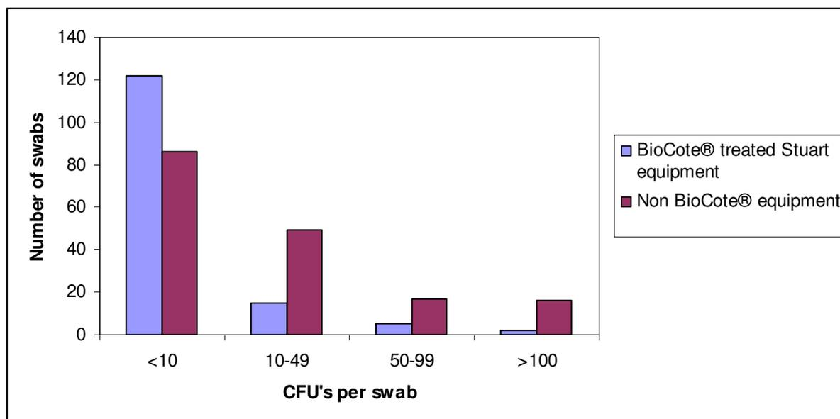
**Figure 1:** Distribution of quantities of total viable bacteria isolated from BioCote®-treated and untreated laboratory equipment.
